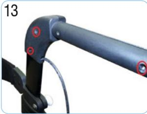
Remove the three screws holding the handle bar housing to the handle bar frame using a Phillips screw driver. Separate the two half's of the brake handle to remove them from the hand bar.
