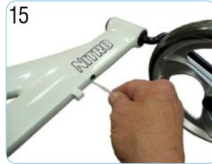
Remove the cord from the old brake and tape the cord to the cable of the new brake. Do not tape the cord to the cable housing. Do not make the taped section wider than the cable housing.
