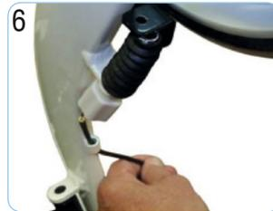
Loosen the cable fastener with a 4mm Allen wrench and remove.
