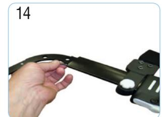
Remove the screw holding the brake handle onto the handle bar using a Phillips screw driver. Remove the brake handle.
