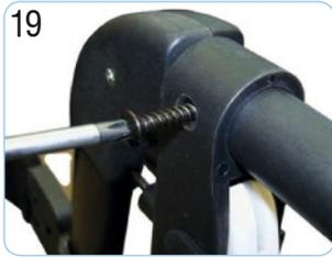
19 Slide the brake handle on to the handle housing. As the brake is slide forward pull on the brake cable coming out of the lower frame. Screw the brake handle in place.
