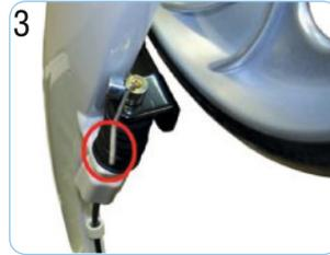
Remove the crimp fitting at the end of the brake cable.
