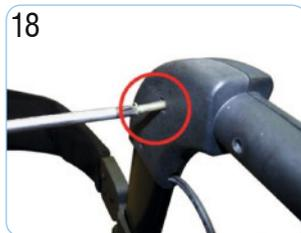
Slide the brake handle on to the handle housing. As the brake is slide forward pull on the brake cable coming out of the lower frame. Screw the brake handle in place.
