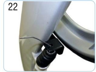
22 Slide the brake cable through the cable adjuster and spring.
