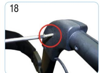
Push the new brake cable down until the brake cable can be seen in the cable hole in the bottom of the frame.
