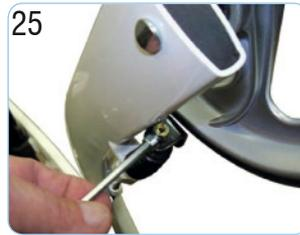
25 Tighten the cable fastener.
