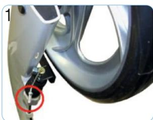
1 Remove the cable-end sleeve from brake wire.
