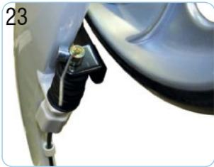
23 Slide the cable fastener on to the cable until the brake blade is about 1/8" from the wheel.
