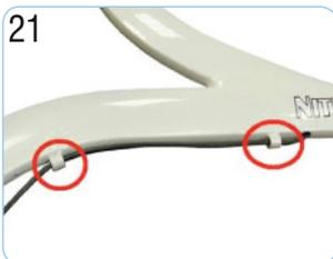
Slide the brake cable through the cable adjuster and spring.
