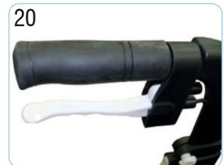
Slide the brake cable through the two lower cable guides.
