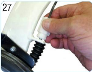
27 Use the cable adjuster to make any needed adjustments to the brake. If the brake can not be adjusted to engage the wheel, loosen the cable faster and re-position as needed.
